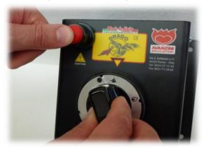
The first firing can be hard when it takes time before the air contained in the Ø 6mm copper tube, which supply the pilot, completely goes away. It is necessary to insist until on the top of the pilot flame all of the 3 flames are on, in order to get a proper ignition of the main burner (see image below).
