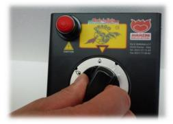
Extract the handle and regulate the high of the flame by acting on the screw (see images below). The right range is when the low flame length is about the half if compared to the long flame length. By turning it clockwise the gas power decreases, by turning it counter clockwise the gas power increases. (In any case when in low flame, the oven must not increase the temperature but maintain it).
