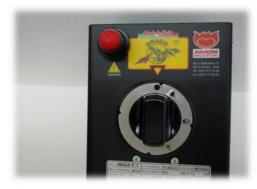
The flame needs to be smooth and silent of yellow colour, but it does not need to colour too much the oven's dome. The air shutter opening regulation can change on the basis of the gas mix used, it usually needs to be placed on the reference N.3 or N.4 (see image below).
