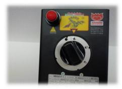
To turn completely off the main gas burner and the pilot flame, you need to place the handle on the black dot (see image below).
